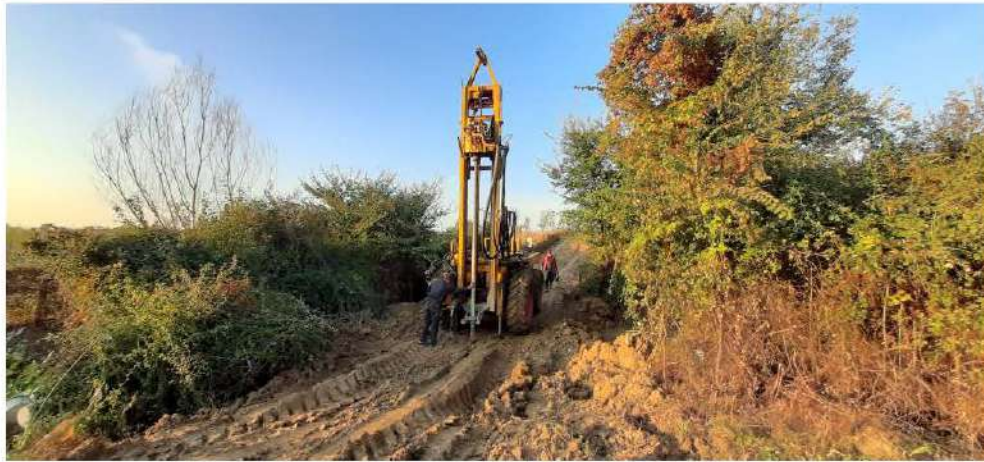
PAGANI PENETROMETER TG 63-200 FOR STATIC AND DYNAMIC PENETROMETRIC TESTS
